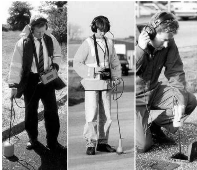
Commonly used listening devices including ground microphones and listening rods (source: Palmer Environmental Limited)
